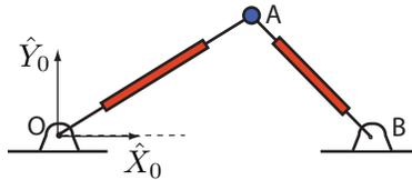
Figure 1: A triangular mechanism, with two linear actuators, OA and AB, which can change lengths  $L_1$  and  $L_2$ .
